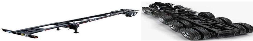
**Flat Bed Trailer:** Cargo pieces loaded on to flatbed trailers must be lashed down to the horizontal flat base of the trailer. These pieces should not be lashed to any side or vertical parts rising from the base of trailer.
