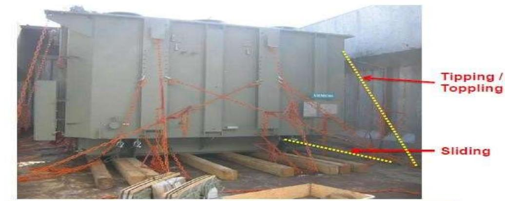
If the cargo has no securing point Loop lashing is the next best method.
