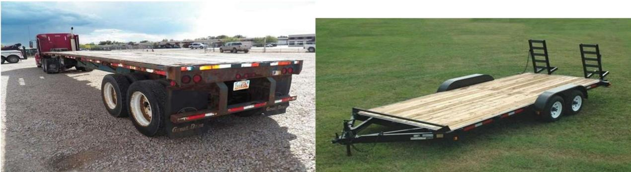
**Flat Bed Truck:** Cargo pieces loaded on to flatbed trucks must be lashed down to the horizontal flat base of the trailer. These pieces should not be lashed to any side or vertical parts rising from the base of trailer.
